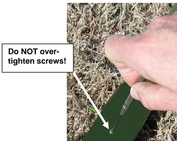
**NOTE:** The antenna should now be fully extended and laying on the ground and all sections should be secured with the stainless steel screws (except the top, tip section which does not require a screw).
