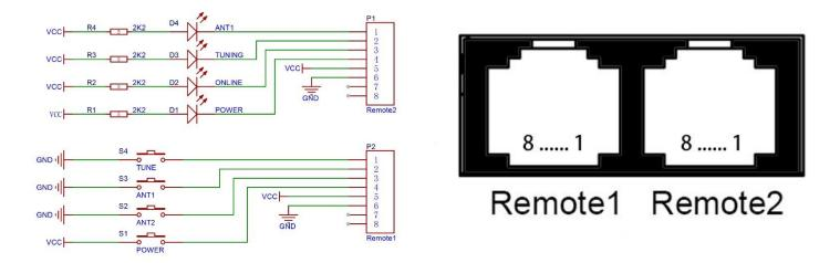
Remote1 and Remote2 are standard RJ45 sockets, and their wiring sequence is shown in the
