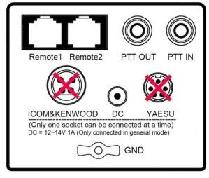
If you use transmitters other than Yaesu, ICOM or Kenwood with an external DC power supply connected, when you press the "POWER" button on the front panel to start, this mode will be set automatically. The voltage of external power supply shall be in the range of 10-15v, and the maximum working current shall not be less than 1A. Other cable connections are described below.
