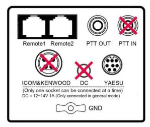
(2) If there is a cable connection between your transmitter and amplifier, please confirm whether this cable contains PTT signal. Usually, this signal is in the first core of the transmitter "LINEAR" socket, or a control cable with two sections of RCA lotus plug. If the PTT signal is included, be sure to disconnect it.
