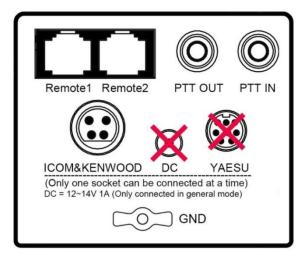
(2) If there is a PTT signal cable between your transmitter and amplifier-- usually this is a cable with lotus plugs at both ends. If the PTT signal cable is concected, be sure to disconnect it.
