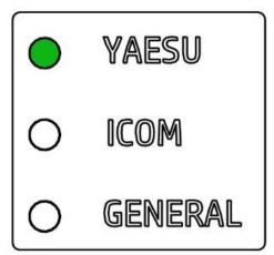
The tuner has three working modes: YAESU mode, ICOM& KENWOOD mode, and GENERAL mode. Users could accomlish one-button operation on the transmitter for maximum automation while using the first two modes.
